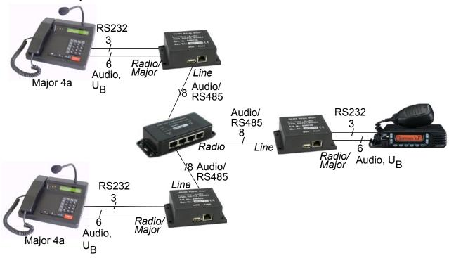
If several control panels are used to control a single radio, the connection is realized with a Distribution Frame DMR. Here, the RS485 lines are connected in parallel.
